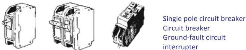
**Ground-fault circuit interrupters (GFCIs)** protect against potentially lethal shock when they detect even minute, but potentially dangerous **ground faults**, or "leaks" of electrical current from the circuit. GFCIs may be incorporated into circuit breakers protecting the entire circuit, outlets protecting everything on the circuit downstream from the GFCI outlet, or as portable devices that can be used at an outlet to give protection for a particular electrical item.
